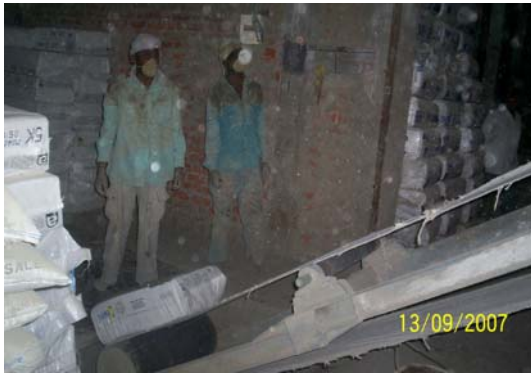
Figure 1:Asbestos fibres bags transported through conveyor belts
