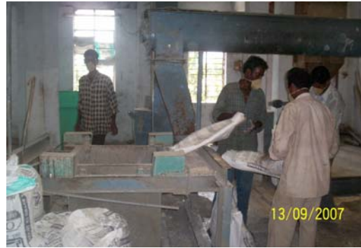
Figure 2:Mixing of asbestos fibres
