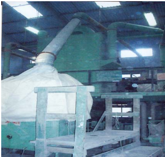
Feeding machine connecting to dust collector
