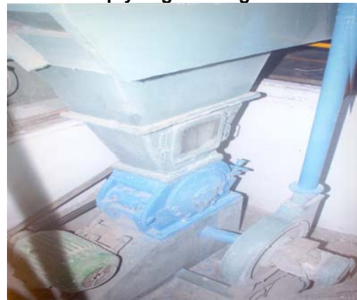
Empty Bags are powdered for Mixing with Fibre
