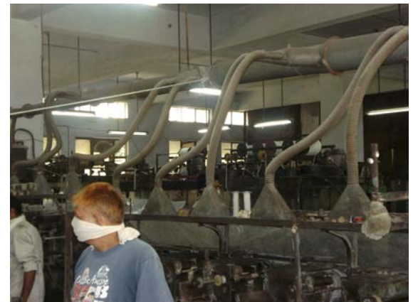
Local Exhaust Ventilation at Winding section
