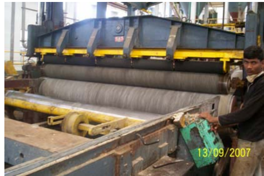
Figure 4:Pipes are being manufactured through continuously laid layers of slurry
