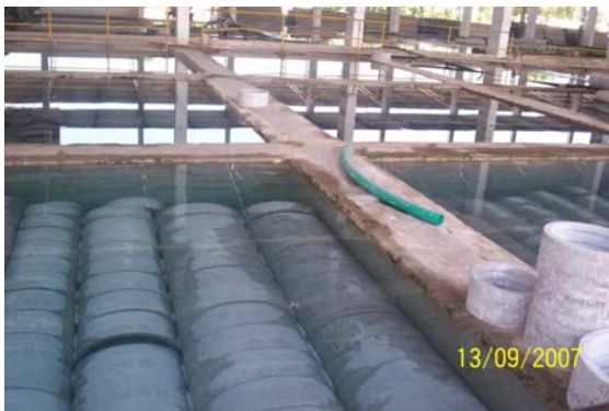
Figure 5:Water curing of manufactured pipes
